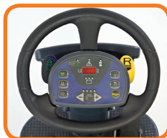
Controls are mounted on the steering wheel for safety
