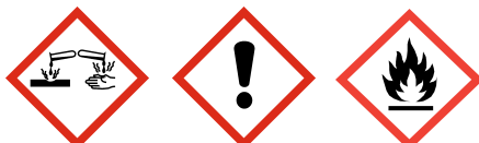
CORROSIVE EXCLAMATION FLAME
